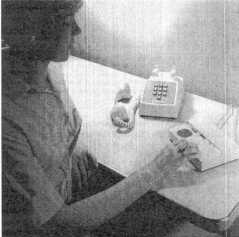
The Code-Com set was another in a long line of devices developed by Bell Telephone Laboratories for use by deaf people. It had three components, a flashing light in the center, with a circular vibrating pad on the left and a sending key, used like a telegraph key, on the right. Property of AT&T Archives. Reprinted with permission of AT&T.
